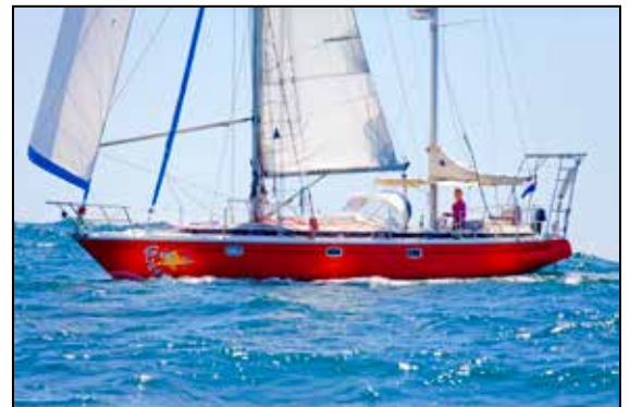
Dekker used a French-built, 40 ft, two-masted Jeanneau Gin Fizz ketch, which Laura named Guppy.
